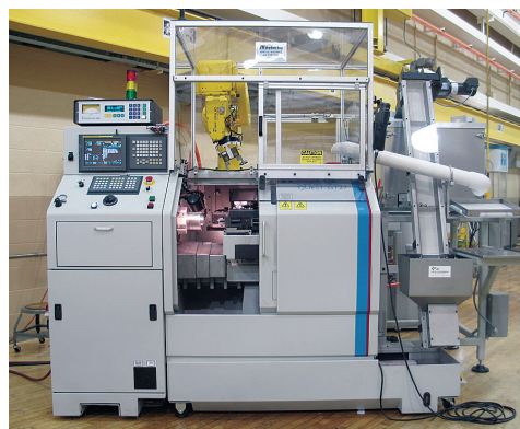
Gang-tool CNC Lathe with internal grinding wheel for fine surface finish requirements. Elevator conveyor drops blanks into bowl feeder to orient parts for robot pickup. In-process gaging.
