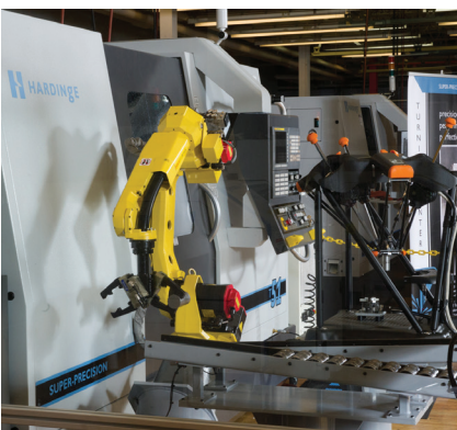
Front cover photo: Hardinge T51 SUPER-PRECISION Turning Center with Fanuc robot and Renishaw comparative gaging.
