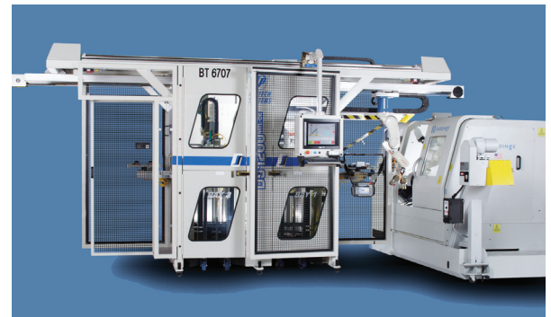
Integrated gantry-style automation system with part staging, washing and post-process gaging systems.
