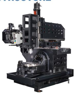
The X/Y/Z axis adopts precision grade roller linear guide rails and heavy-duty sliders to enhance the load-carrying capacity of the transmission system and improve the processing performance of the machine.
