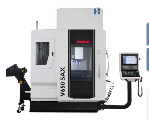
Bridgeport V650 5AX five-axis vertical machining center is developed and designed to meet the processing needs of complex parts in various industries. The large working space and humanized structural design bring users the most convenient experience.
